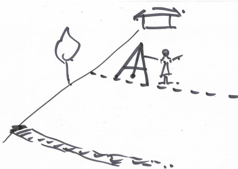
Finding a level line with an A frame. you may 'walk' the A frame along the contour you are exploring, pegging the feet of when ever the plumb line tells you it is level. It is too hard to judge by eye, but your A frame can confirm you have level ground. you repeat this action across the whole line where the Swales will be dug.
